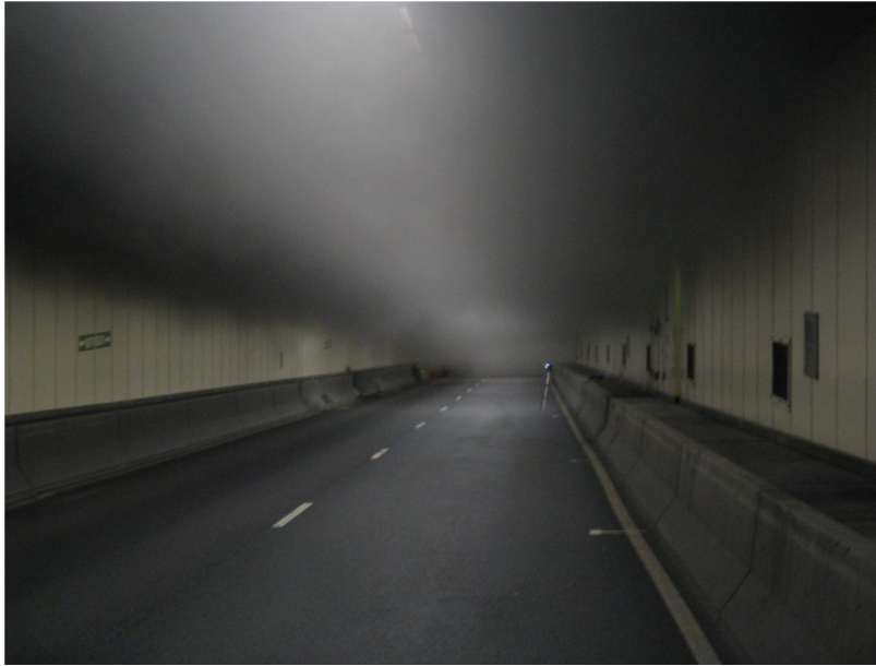
Photograph 5 - Test 2 - stratification of smoke 200m away downstream (to the north) from fire immediately after deluge was shut off.
