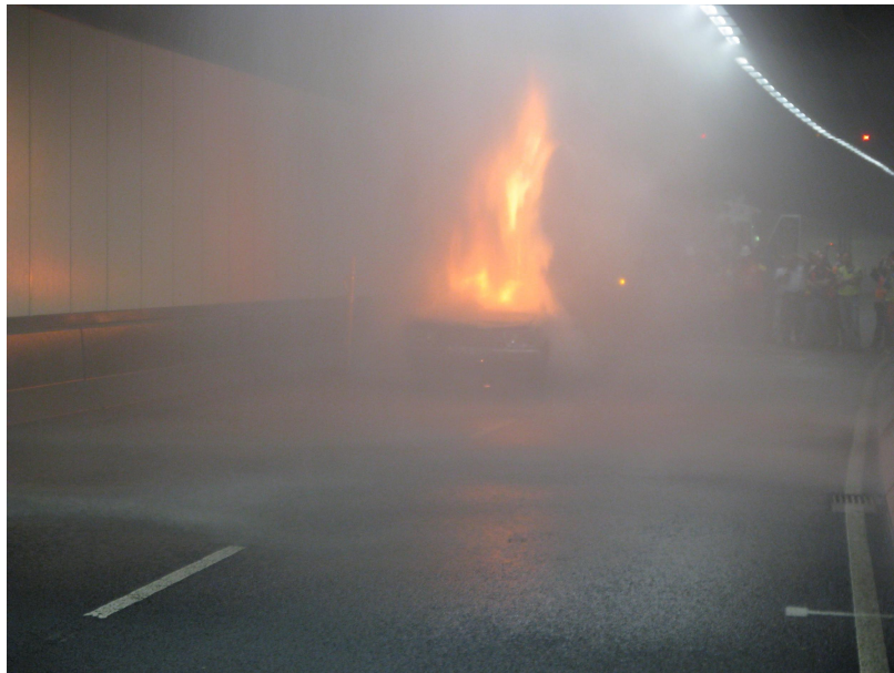
Photograph 4 - Test 1 - visibility after deluge activation (better than 30m). There is no smoke as the damper is directly above the fire.
